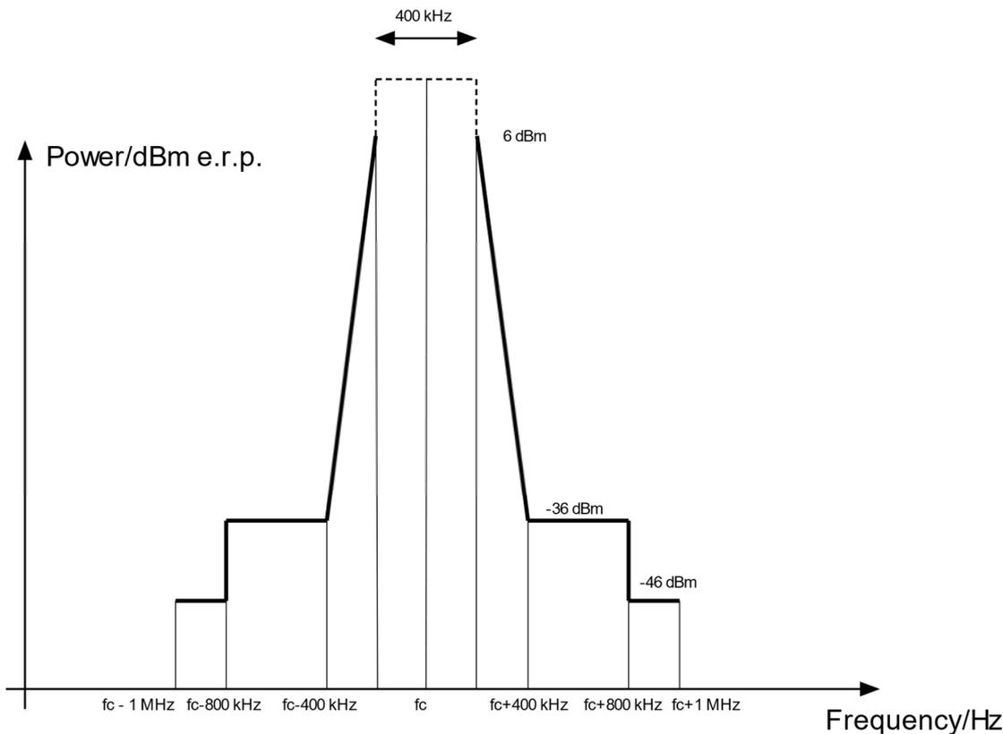
NOTE 1: Where  $f_c$  is the centre frequency of the carrier transmitted by the interrogator applicable over the frequency range  $f_c \pm 1\,000$  kHz.
