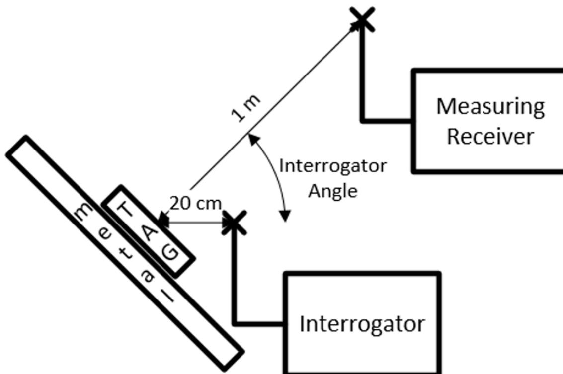
Figure 17: Measurement of tag emissions with metal
