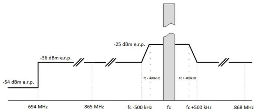
NOTE 1:  $f_c$  is the centre frequency of the carrier transmitted by the interrogator.
