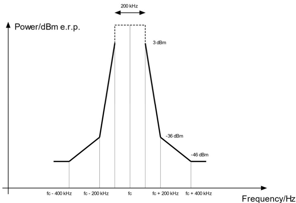
NOTE 1: Where  $f_c$  is the centre frequency of the carrier transmitted by the interrogator applicable over the frequency range  $f_c \pm 500$  kHz.
