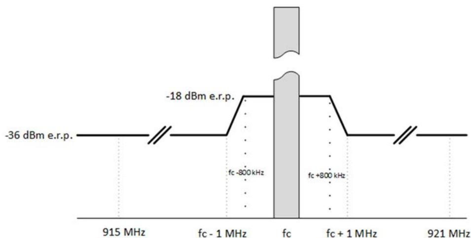
NOTE 1:  $f_c$  is the centre frequency of the carrier transmitted by the interrogator.
