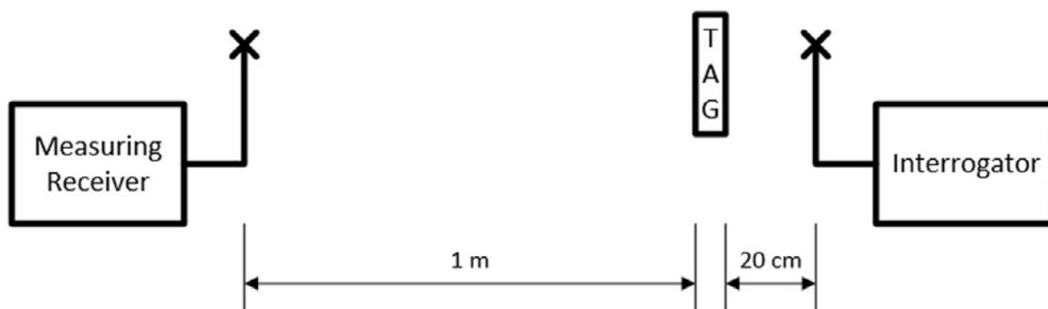
**Figure 16: Measurement of tag emissions**
