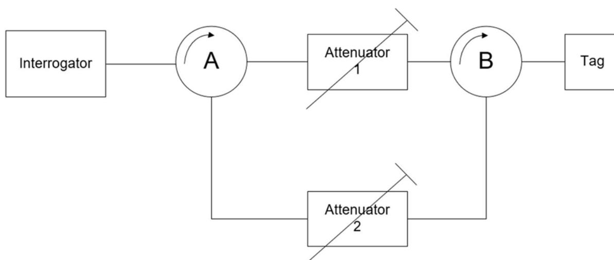
**Figure 12: Conducted test set up for receiver sensitivity**
